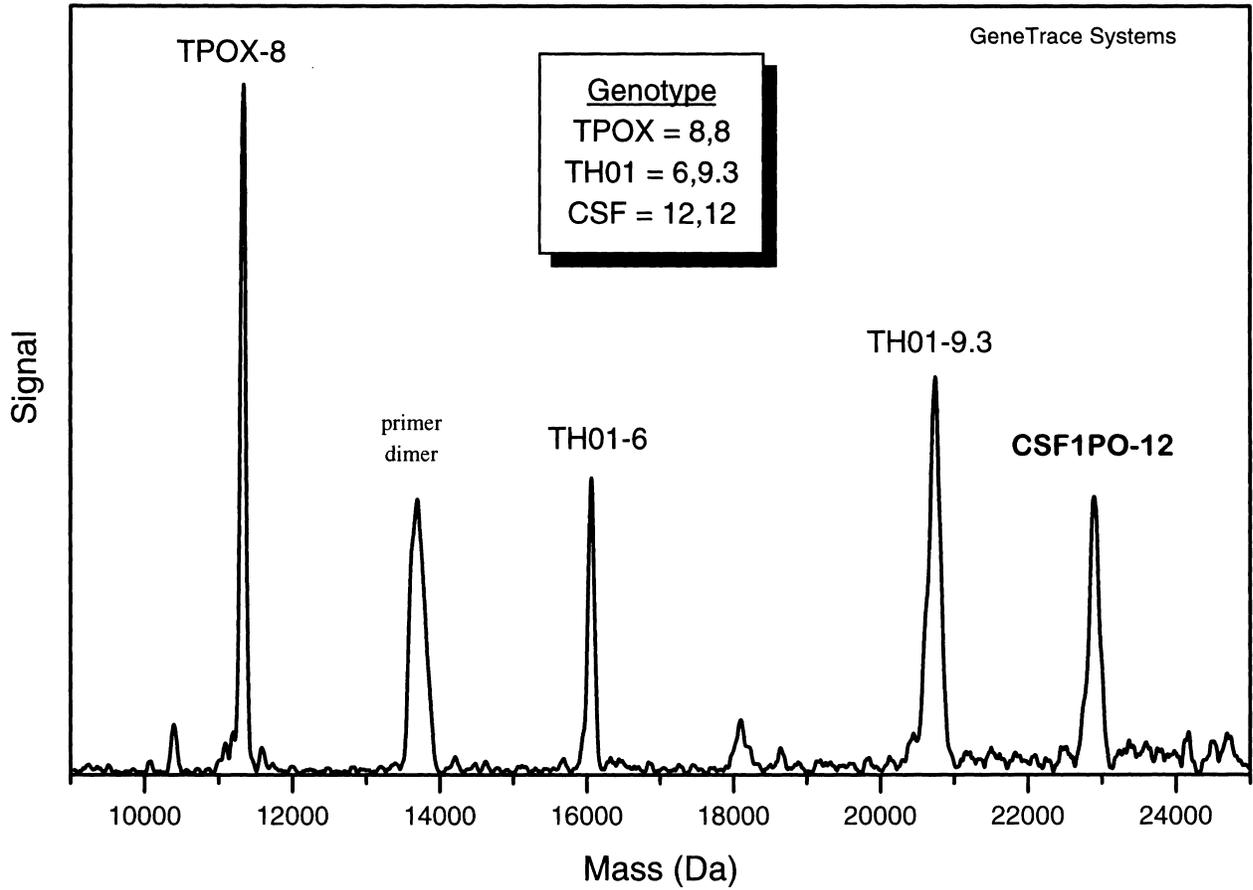
Figure 4 (b) A mass spectrum of a CTT multiplex sample.
