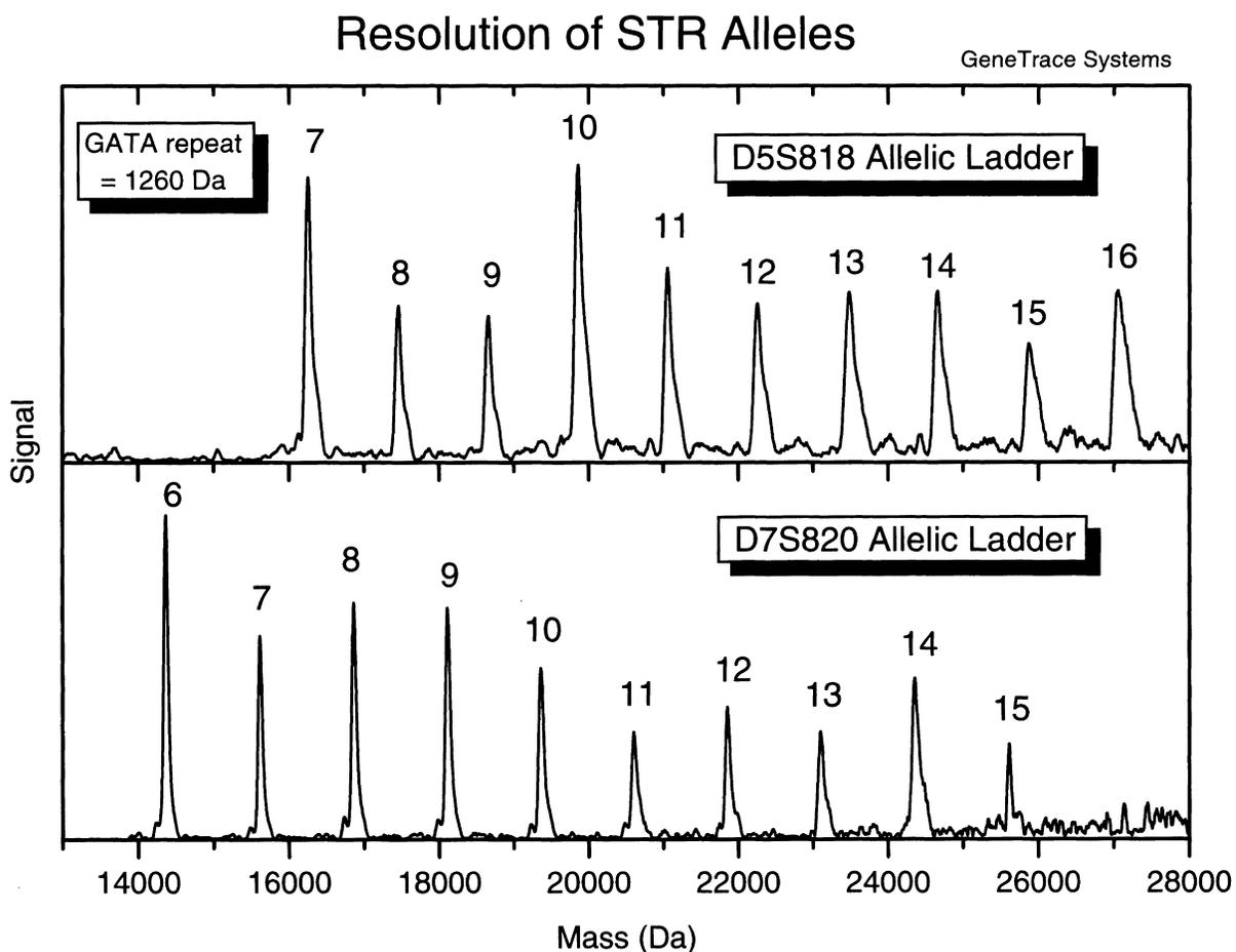
**Figure 3.** Resolution of tetranucleotide STR alleles demonstrated with D5S818 and D7S820 allelic ladders. The allelic ladders were reamplified from diluted PE Applied Biosystems AmpFISTR Yellow allelic ladders using GeneTrace-designed primers and PCR conditions as described in the Materials and Methods section.
