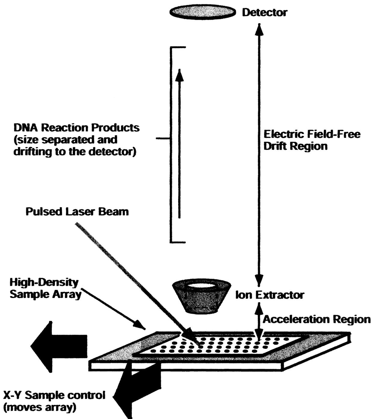
**Figure 1.** Schematic diagram illustrating the principal components of DNA analysis by time-of-flight mass spectrometry. Each STR sample is imbedded within a matrix compound in a ~1-mm diameter spot located on the sample plate. A pulsed laser beam liberates the DNA from the matrix for mass analysis. STR alleles are separated by their time-of-flight to the detector, a process that occurs in a few hundred microseconds.
