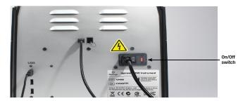
Figure 13. The On/Off switch.
