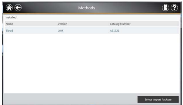
Figure 37. Methods window. This window displays a list of the methods that are currently installed in the Maxwell ® CSC User Interface. Touching the ‘Select Import Package’ displays a file path for navigating to a particular file (Figure 39). This file will be used to import a new or updated method/kit pair.
