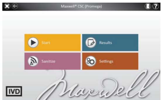
Figure 28. Maxwell® CSC Home screen. Selecting Settings opens the Maxwell® CSC 'Settings' screen from which bar code entry options can be configured.
