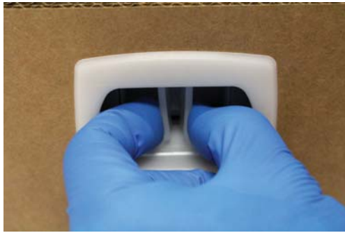
Figure 7. Remove the white plastic clips that lock the shipping container.
