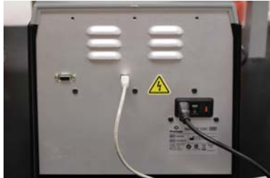
Figure 14. Connect the Tablet PC to the back of the Maxwell ® CSC Instrument.
