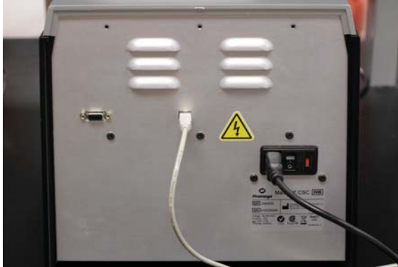
Figure 3. Rear view of the Maxwell® CSC Instrument. The rear of the instrument showing the On/Off switch, power cable connector and USB communication port.
