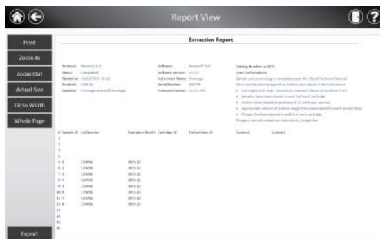
Figure 58. Report View screen. The 'Report View' screen displays the sample tracking and protocol-specific information for the current instrument run. Included in this report are the sample tracking information recorded prior to starting the protocol, the final status of the protocol (Completed or Aborted), the time the protocol run was started, the length of time the protocol took to process, the operator ID and additional instrument information. In the lower left corner of the screen is an Export button that will be used for exporting report information.
