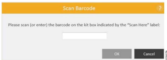
Figure 44. Scan Bar Code screen. Scanning the bar code automatically selects the protocol on the Maxwell® CSC Instrument.
