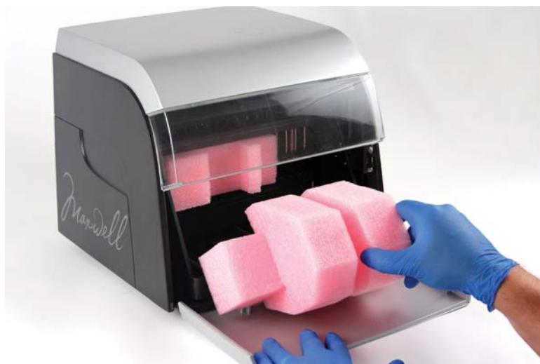
Figure 9. Remove the two foam pieces from inside the instrument.
