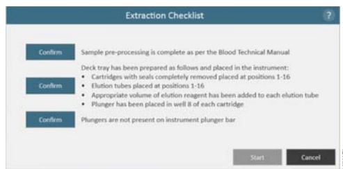
Figure 48. Extraction Checklist screen. This screen indicates the steps that will need to be performed to prepare the instrument for processing the selected samples. Preprocessing steps are not indicated on the 'Extraction Checklist' and should be performed prior to this stage according to the technical manual for the kit being processed.
