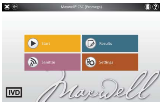
Figure 65. Home screen. Selecting the Sanitize button begins the process of Sanitizing the Maxwell® CSC Instrument.
