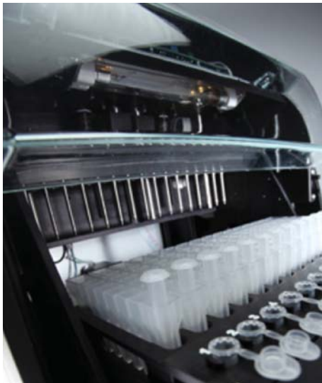
Figure 4. Magnetic assembly components and platform. The hardware components inside the Maxwell® CSC Instrument. The magnet and plunger bars, which are used for sample processing, and the platform containing the deck tray are evident.
