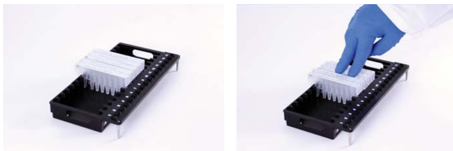
Figure 49. Place the cartridges in the deck tray, and press firmly to snap them in place.
