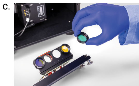
Figure 18. Panel A. Removing the front panel. Panel B. Filter slide panel. Panel C. Removing emission filters.
